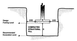
Overexcavation / Backfill NOTE: Excavations in sketches shown vertical for
