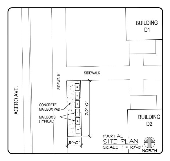
INSTALL CONCRETE MAILBOX PAD. 5'-O"  $\times$  20'-O"  $\times$  6" THICK 4000 P.S.I. AND (5) CLUSTER MAILBOX UNITS AND (I) PARCEL BOX, ALL ON PEDESTALS. PEDESTALS BOLTED TO CONCRETE PAD WITH (4) I/2-I3 ANCHOR BOLTS.
